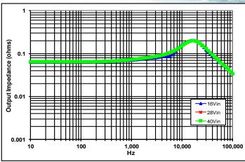
Figure 26: Magnitude of incremental output impedance of -12V output (-Zout = -vout /-iout) for minimum, nominal, and maximum input voltage at full rated power.
