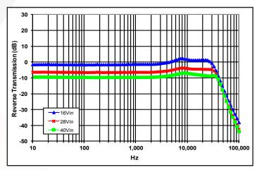
Figure 30: Magnitude of incremental reverse transmission from -12V output (-RT = iin /-iout) for minimum, nominal, and maximum input voltage at full rated power.
