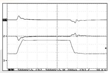
Figure 19: Output voltage response to step-change in input voltage (16V - 50V - 16V). Load cap: 10μF, 100mΩ ESR tantalum cap and 1μF ceramic cap. Ch 1: +Vout (500mV/div); Ch 2: -Vout (500mV/div); Ch 3: Vin (20V/div).
