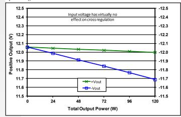
Figure 10: Load regulation vs. total output power from zero to to full load where -lout equals three times +lout at nominal input voltage and Tcase = 25°C.
