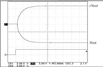
Figure 15: Turn-on transient at full rated load current (resistive load) (5ms/div). Input voltage pre-applied. Ch 1: +Vout (5V/div); Ch 2: -Vout (5V/div); Ch 3: Enable2 input (5V/div).
