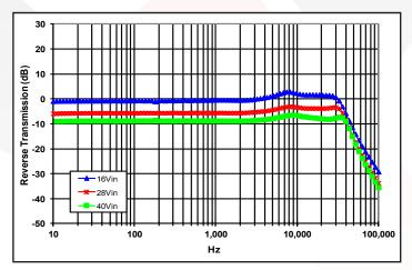
Figure 29: Magnitude of incremental reverse transmission from +12V output (+RT = iin /+iout) for minimum, nominal, and maximum input voltage at full rated power.
