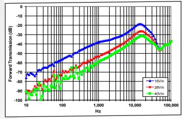
Figure 28: Magnitude of incremental forward transmission of -12V output (-FT = -vout /vin) for minimum, nominal, and maximum input voltage at full rated power.
