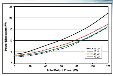
Figure 2: Power dissipation vs. output power, from zero load to full load with equal load on the +12V and -12V outputs at minimum, nominal, and maximum input voltage at 25°C.
