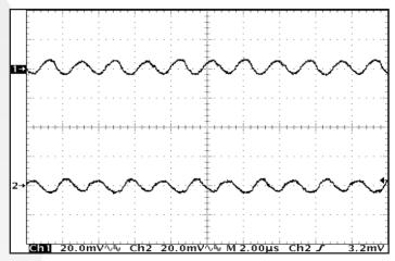
Figure 22: Output voltage ripple, +Vout (Ch 1) and -Vout (Ch 2), at nominal input voltage and full load current evenly split (20mV/div). Load capacitance: 1µF ceramic cap and 10µF tantalum cap. Bandwidth: 10MHz. See Figure 20.
