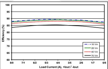
Figure 3: Efficiency vs. output current, with total output current fixed at 80% load (96W) and loads split as shown between the +12V and -12V outputs at minimum, nominal, and maximum input voltage at 25°C.
