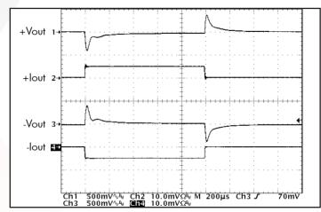
Figure 18: Output voltage response to step-change in total load current (0%-50%-0%) of total lout (max) split 50%/50%. Load cap: 1μF ceramic cap and 10μF, 100 mΩ ESR tantalum cap. Ch 1: +Vout (500mV/div); Ch 2: +Iout (5A/div); Ch 3: -Vout (500mV/div); Ch 4: -Iout (5A/div).
