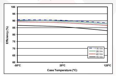
Figure 5: Efficiency at 60% load (3A load on +12V and 3A load on -12V) versus case temperature for Vin = 16V, 28V, and 70V.
