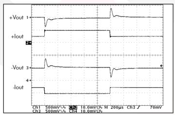
Figure 17: Output voltage response to step-change in total load current (50%-100%-50%) of total lout (max) split 50%/50%. Load cap:  $1\mu$ F ceramic cap and  $10\mu$ F, 100 m $\Omega$  ESR tantalum cap. Ch 1: +Vout (500mV/div); Ch 2: +Iout (5A/div); Ch 3: -Vout (500mV/div); Ch 4: -Iout (5A/div).
