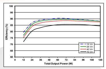
Figure 1: Efficiency vs. output power, from zero load to full load with equal load on the +12V and -12V outputs at minimum, nominal, and maximum input voltage at 25°C.
