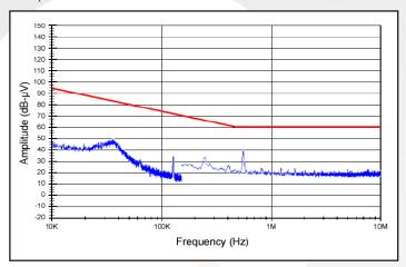
Figure 33: High frequency conducted emissions of MQFL-28-05S, 5Vout module at 120W output with MQME-28-P filter, as measured with Method CE102. Limit line shown is the 'Basic Curve' for all applications with a 28V source.
